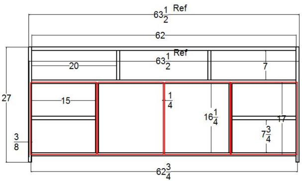
Note: Reference is used because the wood thickness is considered 3/4".
